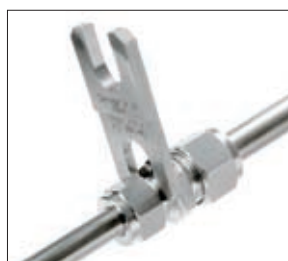
Properly tightened, the gauge will not fit
